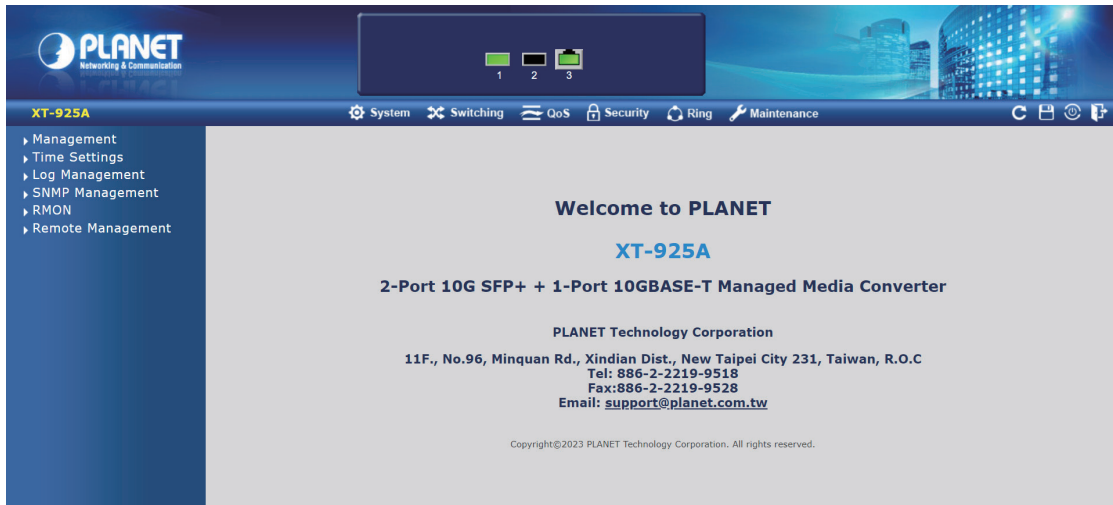
Figure 3-3: Web Main Screen of Managed Media Converter (Use XT-925A as a representative)
